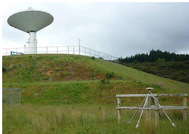
Figure 10. Collocated space geodesy facilities: the GNSS base station WARK and the IVS network station WARK12M (12m radio telescope)
